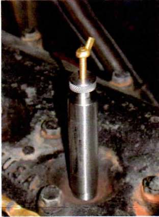
Indicator Installed with Ear pointing towards Piston
